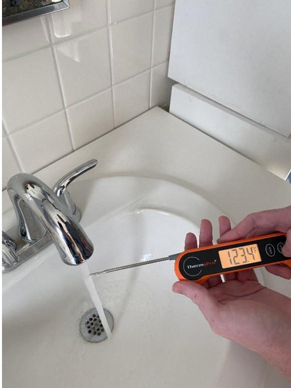
Photograph 11: All-purpose thermometer registering a water temperature of 123.4° F.
