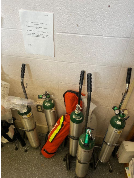
Photograph 8: Stored oxygen tanks were not clearly distinguishable as full or empty.
