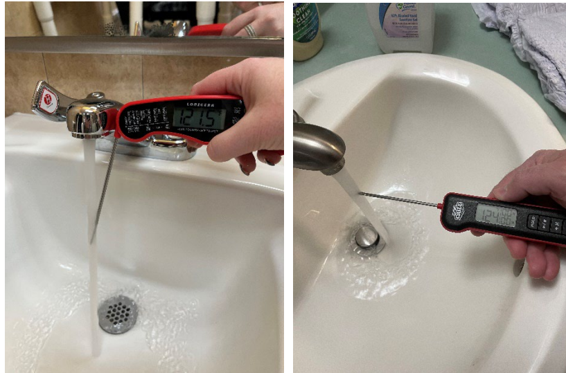
Photograph 11 (left): All-purpose thermometer registering a water temperature of 121.5 °F.
